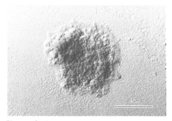
Figure 8. Single crystal obtained from toluene extraction of a 5% gel in 1-chloroundecane (quenching temperature -15 °C) annealed 6 days at 20 °C.
